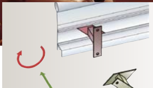
Quick suspension of the frame on its mounts and locking feature by 45° rotation
